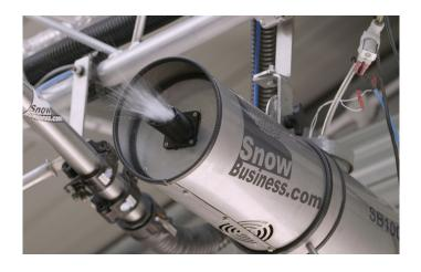
"With the Ultimaker, I can print a nozzle in 7 hours, I can test it, make a small adjustment and print another one. There's also a huge cost difference between outsourcing this and doing it myself. In-house 3D printing cost me a couple of euros worth of plastic whereas with outsourcing it was £125 every time I wanted to make a design change."
