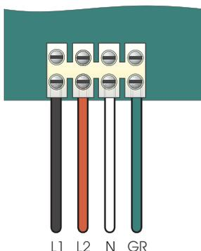
The following instructions must be followed for a permanently connected equipment module designed to operate at 240 Volts. The heater will provide 4500 watts (4.5kw) of heat when the pump is on low speed and the thermostat is calling for heat.
