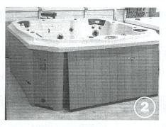
Position a side panel under spa lip with black kickboard on the bottom overlapping cabinet corner. Long panels will match up with long sides of spa. Make sure bolt holes line up, you may have to rotate the cabinet corner 180° (top to bottom).
