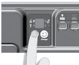
Press select button to select the proper phase configuration setting.
