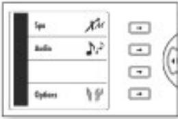
This menu allows control of all pumps, blower and spa light, as well as the activation of the Economy and Standby modes. Every time a device is on, its animated icon is displayed. All pump activity can be stopped at once by activating the Standby mode.
