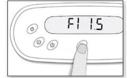
**IMPORTANT:** To reset the first filter cycle start time, skip step 5 and continue pressing the *Light* button until the actual temperature is displayed. Powering down of the spa will also reset the first filter start time.
