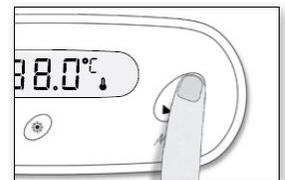
The "heater" indicator lights up when the heater is on. It flashes when there is a request for more heat, but the heater is not on. Once set temperature is reached the indicator shuts off and the low speed of the jet pump turns off after 30 seconds (if not in filter cycle).
