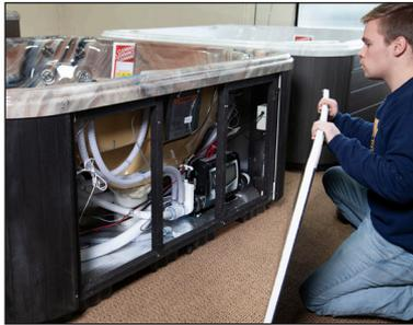
Remove the spa panel for access to spa components. Reverse these steps to reattach the spa access panel.
