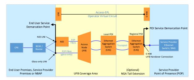
Enhanced Bitstream 4 service, with and without Tail Extension. It is not intended to represent every situation or detailed physical architecture. The following points should be noted:
