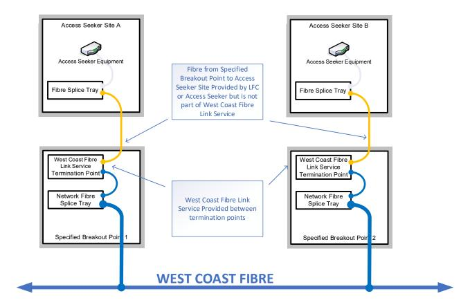
This is a generic diagram showing the standard configuration and Service Demarcation Points. It is not intended to represent every situation or detailed physical architecture and the LFC reserves the right to use or require other physical architecture. The following points should be noted:
