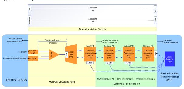
This is a generic diagram showing the standard configuration and Service Demarcation Points. It is not intended to represent every situation or detailed physical architecture.
