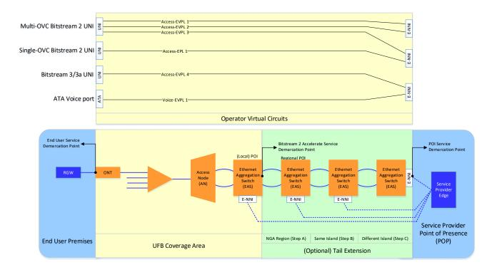
This is a generic diagram showing the standard configuration and Service Demarcation Points. It is not intended to represent every situation or detailed physical architecture. The following points should be noted:
