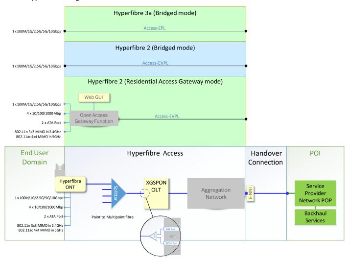
This is a generic diagram showing the standard configuration and Service Demarcation Points. It is not intended to represent every situation or detailed physical architecture. The following points should be noted:
