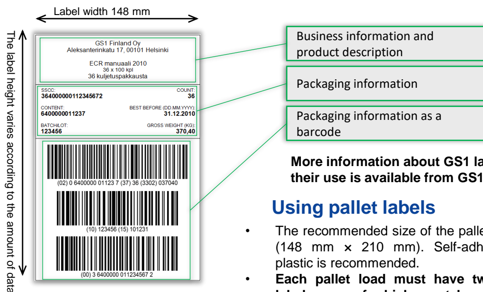
Pallet label in accordance with the GS1 ELL standard PALLET LABEL (European Logistic Label)
