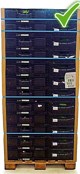
An example of how to tie a fruit/vegetable pallet.
