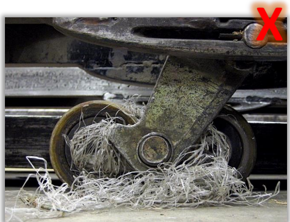
A nylon net wrapped around forklift wheels.
