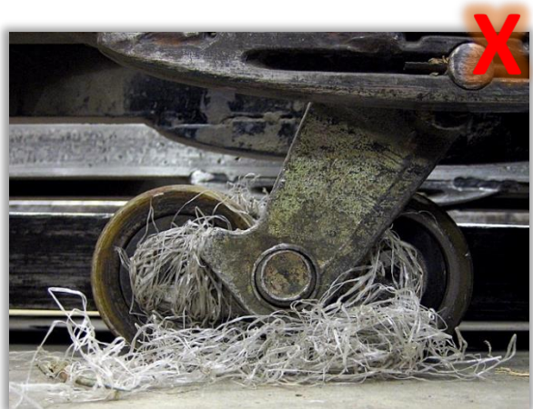
A nylon net wrapped around forklift wheels.
