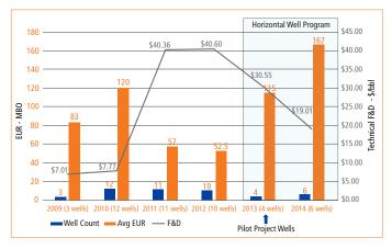
Figure 3. The diminishing returns of a vertical exploitation program as compared to horizontal multi-stage program in Turkey's Şelmo field.
