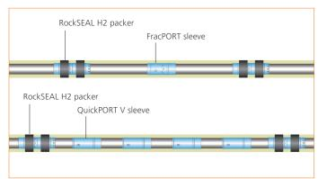
Figure 1. Single entry StackFRAC and limited entry QuickFRAC open hole multi-stage completion systems used for acid stimulation of pilot wells.
