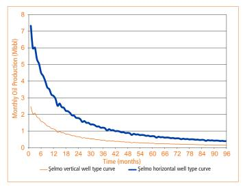
Figure 2. Comparison of vertical and horizontal wells type curves in Selmo field.
