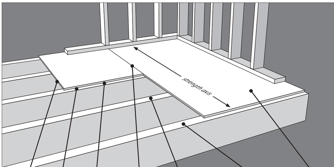
Tongue and groove edges (or 2" lumber blocking between supports)
