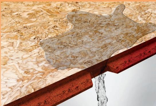
The RainChannel<sup>®</sup> self-draining notch system—utilized in every LP TopNotch solution—allows water to drain quickly from the surface. Combined with a moisture-resistant edge seal, the RainChannel system helps fight moisture absorption and edge swell, reducing the need for sanding.
