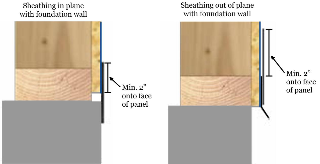
Note: LP WeatherLogic Seam & Flashing Tape must extend at least 2” onto the face of the LP WeatherLogic panel. LP does not require the tape to adhere to the masonry foundation.
