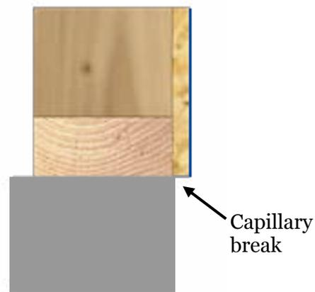
Note: Install a capillary break between the foundation and sill plate as required by code.
