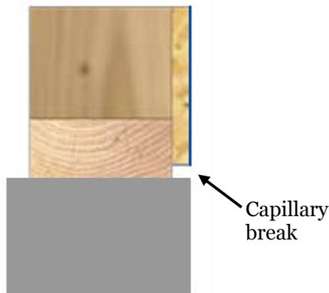
Sheathing out of plane with foundation wall
