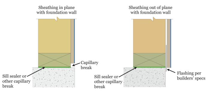
Note: Install a capillary break between the foundation and sill plate as required by code.
