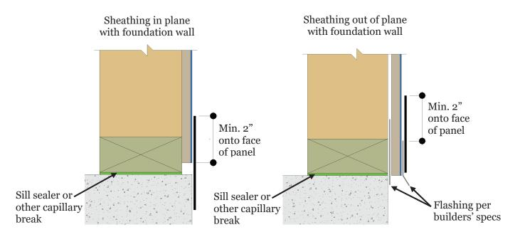
Note: LP WeatherLogic Seam & Flashing Tape must extend at least 2" onto the face of the LP WeatherLogic panel. LP does not require the tape to adhere to the masonry foundation.
