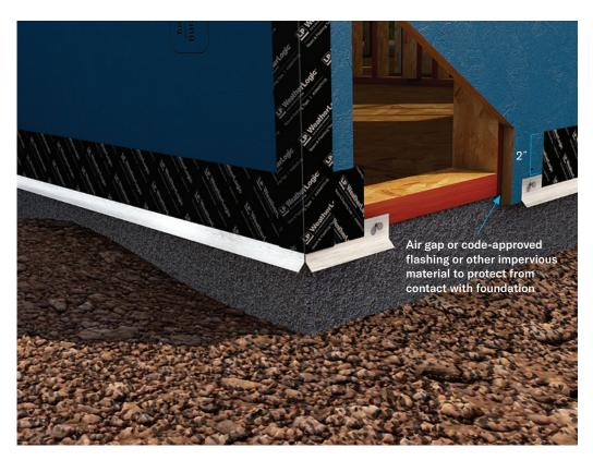
NOTE: This figure depicts just one possible detail. A drip edge or other means of flashing at the transition, if used, should follow local code and approved project specifications.
