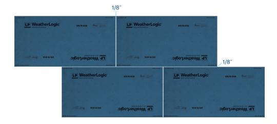
• Provide 1/8" space between all panel ends and edges. Use a spacer tool (e.g., a 10d box nail) to ensure accurate and consistent spacing.
