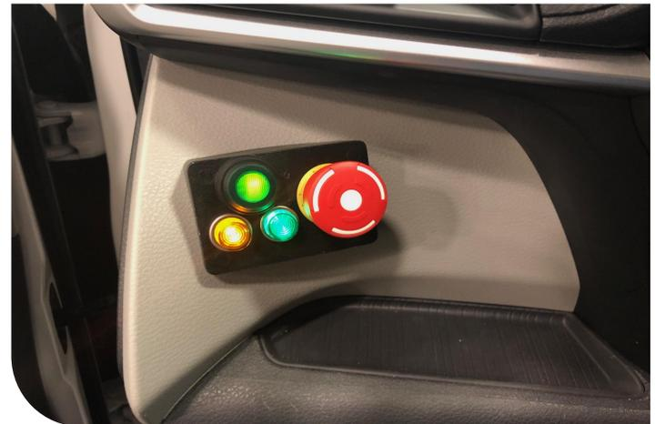
The Driver shutoff button is located to the left of the steering wheel.
