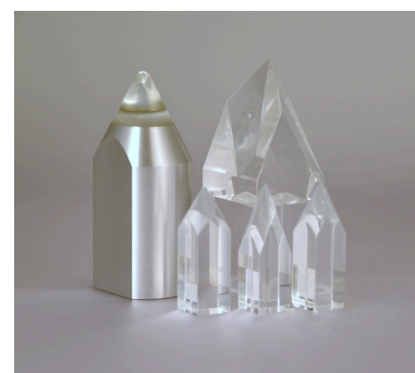
Figure 3.19: Scale models (on two different scales) of different styli. The example on the left is bonded, the other four are nude.
