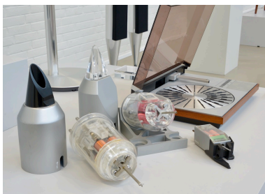
Figure 3.5: Large-scale models of the MMC cartridges used for past demonstrations.
