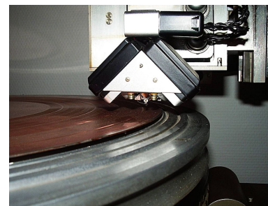
Figure 3.10: A Neumann-Teldec cutting head creating the groove in the master disc. The cutting stylus shown in Figure 3.9 can be seen just under the circular support under the head. (Wikimedia Commons)
