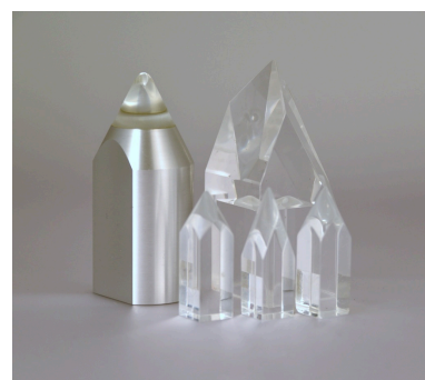
Figure 3.18: Scale models (on two different scales) of different styli. The example on the left is bonded, the other four are nude.
