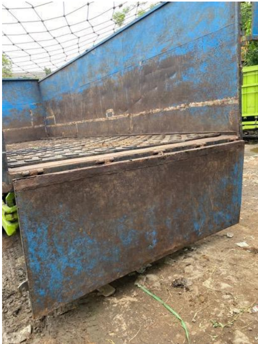
Images: Truck tailgate (left) and floor (right) prior to mat installation, showing use of coconut husk for bedding and traction.
