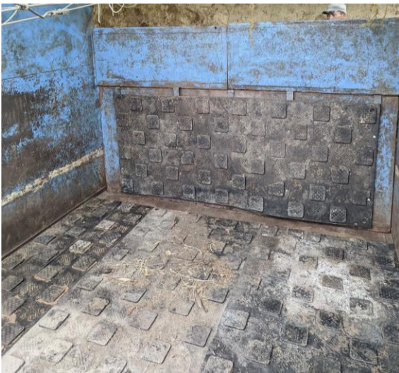
Images: Rubber matting temporarily installed on truck tailgate (left) and floor (right).
