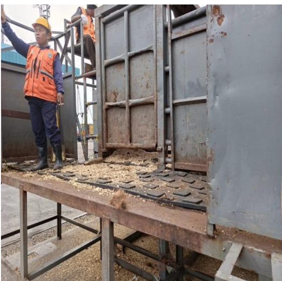
Images: Discharge platform following YoungStar rubber mat installation.
