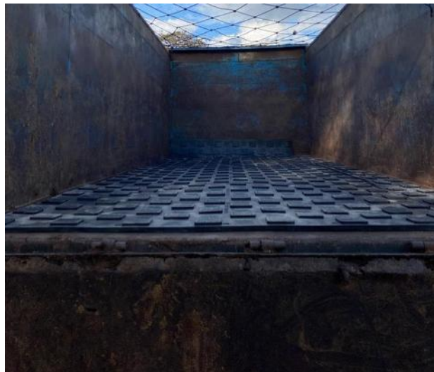
Images: Rubber matting temporarily installed on truck tailgate (left) and floor (right).
