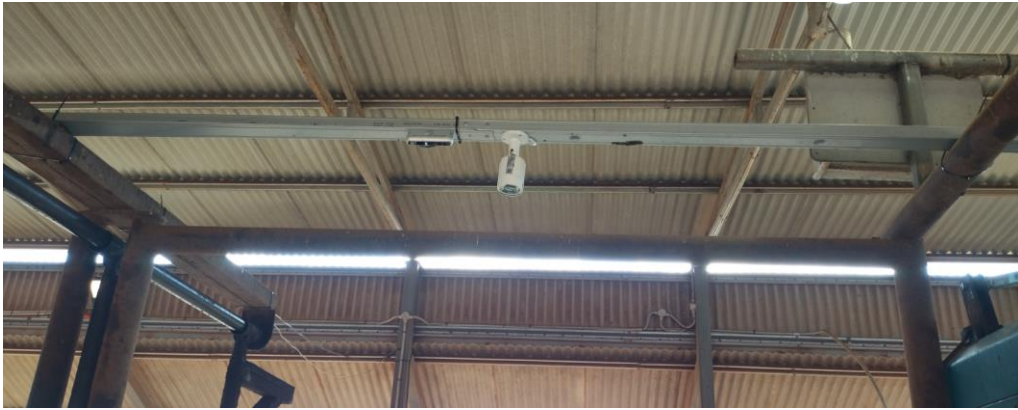
Figure 4: Temporarily mounted 3D (left) and RGB (right) cameras
