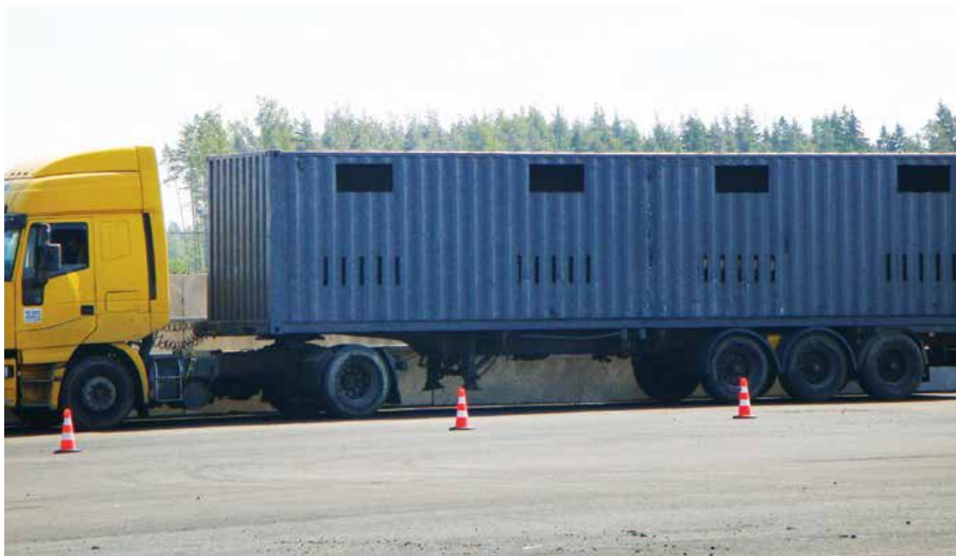
Figure 4.15. Live cattle transport trailers converted from shipping containers. Source: ExpoTrade.
