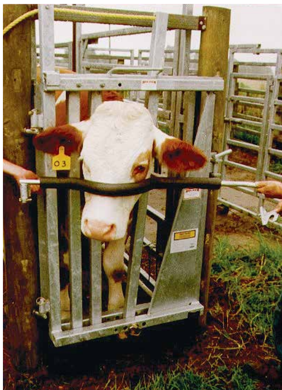
Figure 2.31. A head bail may be installed at the end of a race instead of a crush, but it has limited functionality, and is best suited for small cattle herds. Source: Holdem Cattle Handling Equipment.
