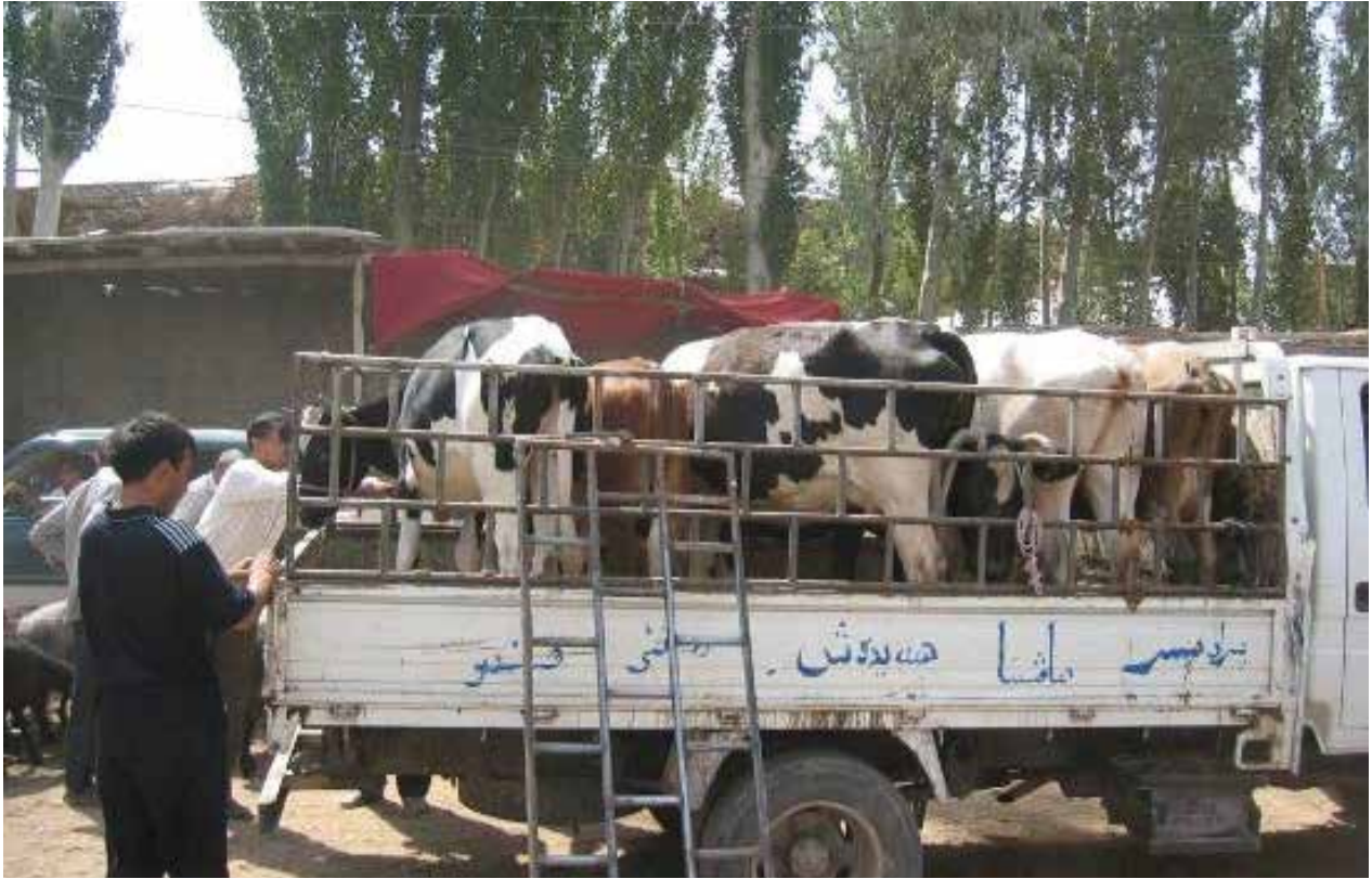
Figure 4.13. Sides of this truck are too low, and there is not a sufficient visual barrier to discourage animals from trying to escape. Source: Anon.
