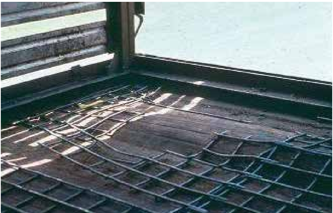
Figure 4.12. Reinforcing mesh is too light for use as truck flooring and can break and cause injuries. Source: LiveCorp and Meat & Livestock Australia.
