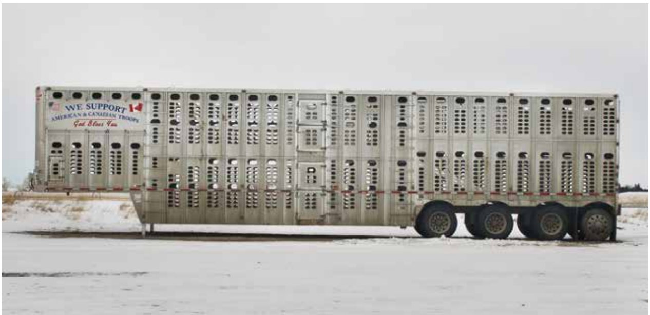
Figure 4.14. A purpose-built live cattle transport trailer providing both ventilation and, with side boards fitted to close off external vents in winter, protection against extreme temperatures. Source: International Agriculture for Development.
