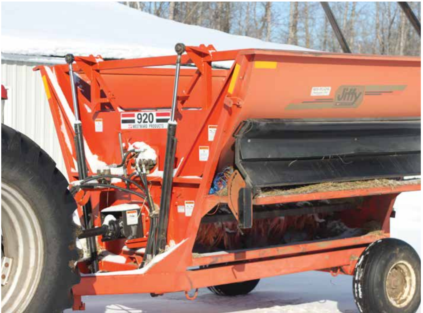
Figure 7.5. Bale processors can be used to add straw for bedding in yards or at winter feeding and shelter sites. Source: International Agriculture for Development.
