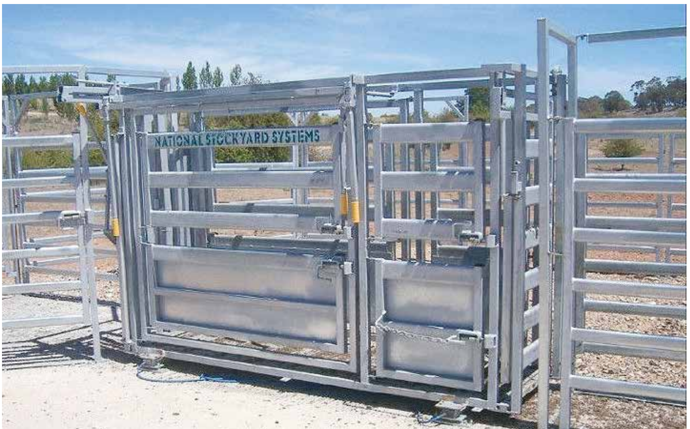
Figure 2.29. Weighing load bars installed under a cattle crush equipped with an internal floor. Source: National Stockyard Systems.
