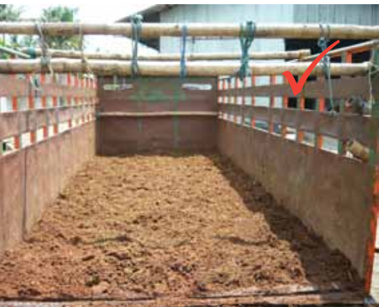
Slippery truck floors should be covered with bedding.
