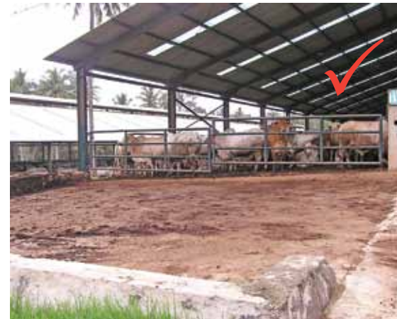
Well-designed feedlot with shelter from sun and rain and with good ventilation
