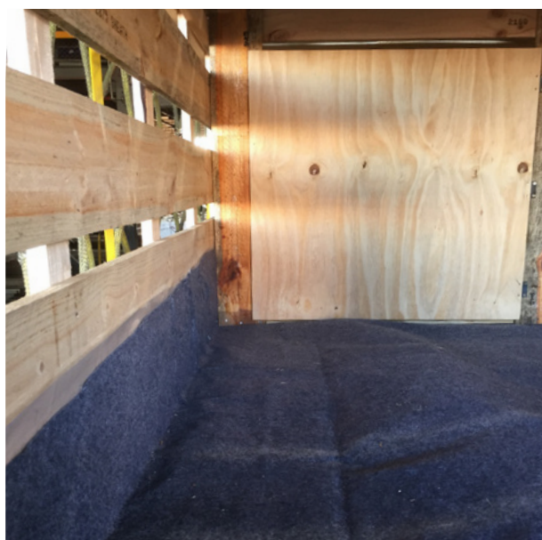
Figure 18. Carpet over the crate floor, to absorb moisture and provide a non-slip floor surface.
