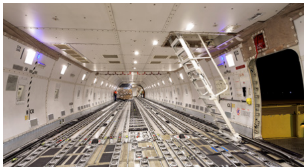
Figure 10. 747-400F main deck looking aft. The ladder goes to the flight deck above. The door on the right provides access for personnel. Freight is loaded onto the main deck through a rear cargo door or nose cone.
