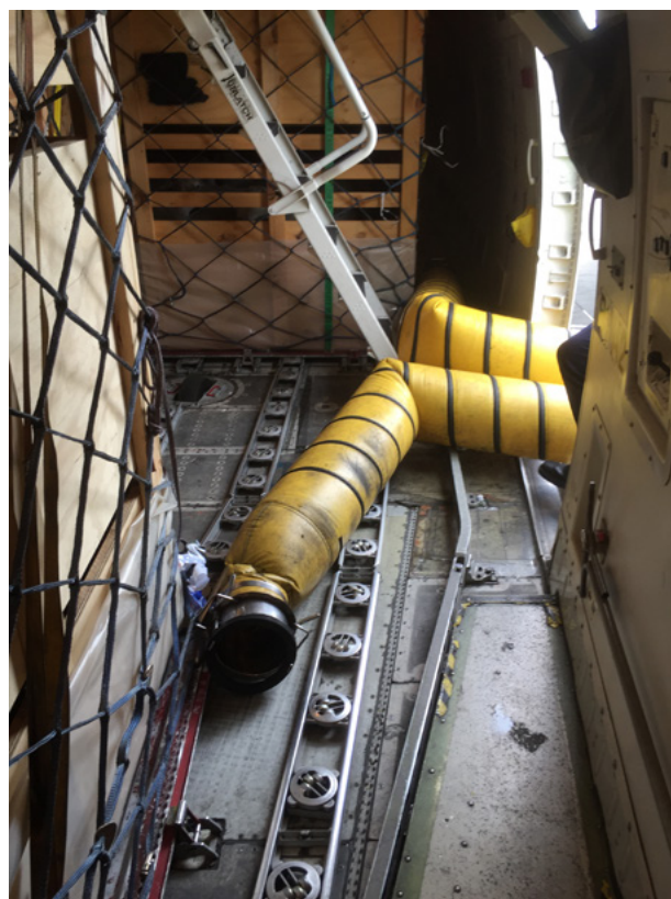
Figure 48. Air pumped onto the main deck to enhance ventilation during a short transit stop.
