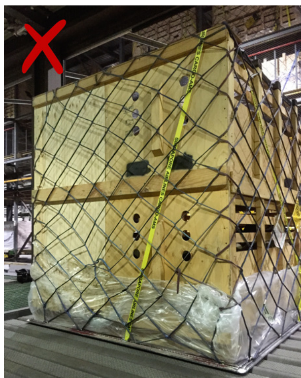
Figure 31. The plastic waterproof barrier between the crate and pallet extends too high, blocking the lower ventilation openings and preventing airflow across the base of this crate.
