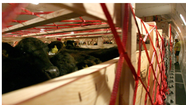
Figure 16. Animals standing normally must not touch the overhead crossbars or cargo net. If the crate has solid sides, they must not extend above head height and there must be ventilation openings in the lower half of the crate on all sides.
