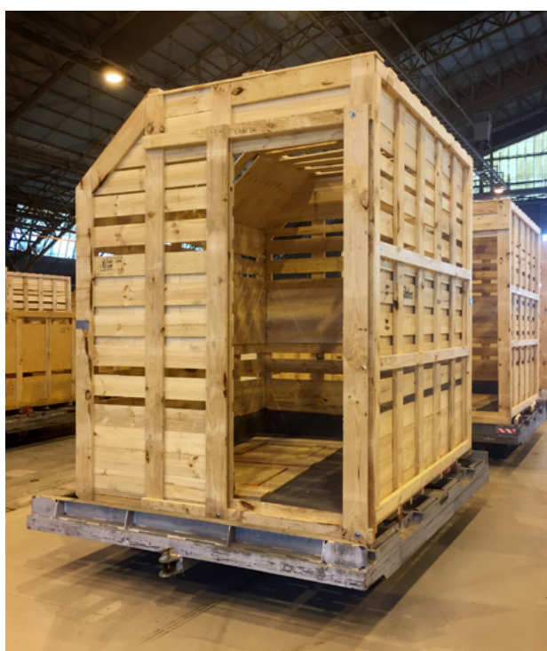
Figure 26. Camel crate. A single-deck 300 cm high crate with full length door.
