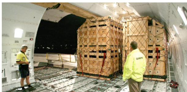
Figure 11. Contoured double-deck cattle crates being loaded on the main deck of a 747-400 freighter through the rear cargo door.
