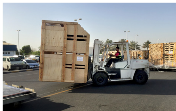
Figure 54. A double-deck cattle crate being moved by forklift. With the cargo net taken off and pallet base removed, the crate must be handled with great care.
