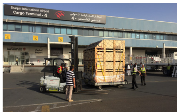
Figure 53. A double-deck cattle crate about to be lifted onto a nearby flat-top truck. Note the extended forklift tines essential for reaching the full width of the crate.
