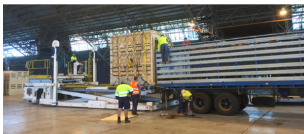
Figure 34. Docking platform for transfer of livestock from truck to aircraft crate – in a disused hanger that provides protection from the weather and is a secure area in the unlikely event of an animal escaping.
