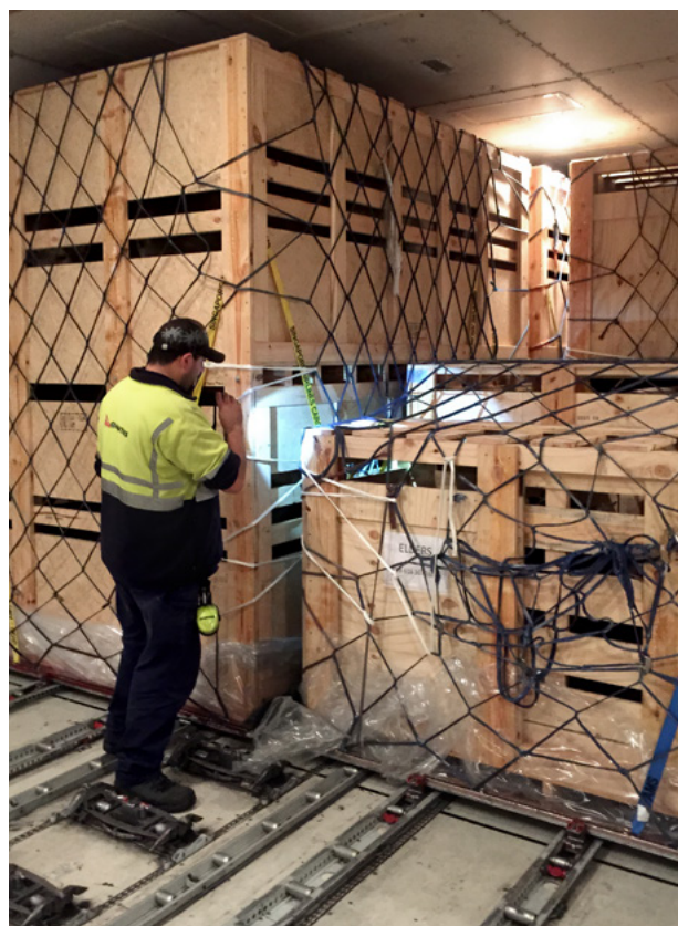
Figure 41. Air flow is enhanced if multi-deck floor to ceiling crates are interspersed with lower crates or empty pallet positions.
