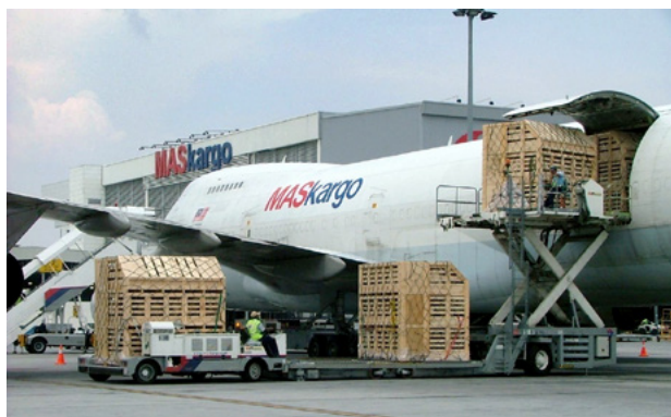
Figure 8. Unloading livestock crates from the main deck of a 747-400 freighter.
