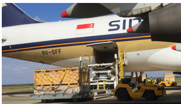
Figure 12. Loading cattle into the aft lower deck hold on a 747-400 freighter.
