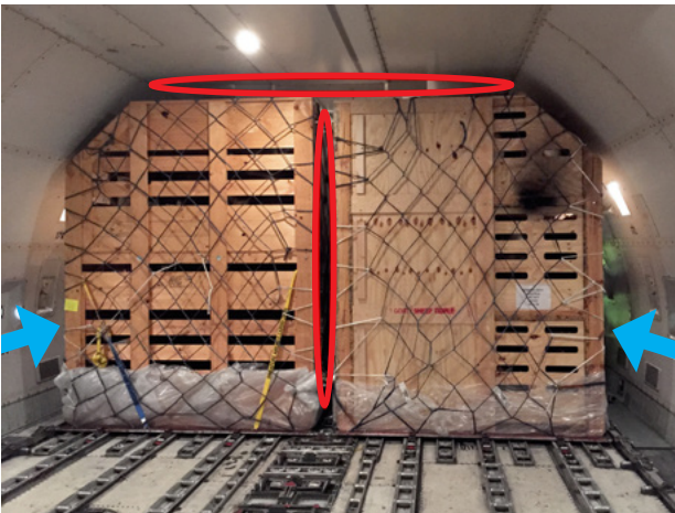
Figure 46. With a block of ceiling high crates, air flow is channelled down the sides of the aircraft hold (blue arrows), producing hot spots (red circles) between crates in the centre of the aircraft and at the ceiling. The temperature in these areas can be a couple of degrees hotter than at the outer sides of the crate. Where possible, multi-deck floor to ceiling crates should be interspersed with lower crates or empty pallet positions.
