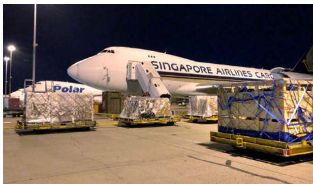
Figure 40. If livestock are loaded with other mixed cargo, the other cargo must not be positioned so as to restrict air flow over or through the livestock crates.
