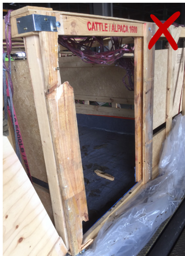
Figure 39. This cattle crate door frame was broken when the exporter tried to take an animal out of the crate, back into a truck. The cattle had not been pre-weighted and drafted into crate lots. There was much wasted time and unnecessary stress on the cattle and the crate could not be adequately repaired on the day of export.
