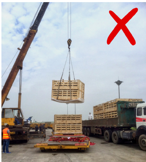
Figure 52. Double-deck sheep crates being lifted by crane. This is a high-risk method of crate handling. Without spacer bars, the crane straps put inward pressure on the crossbars at the top of the crate, which are likely to break.
