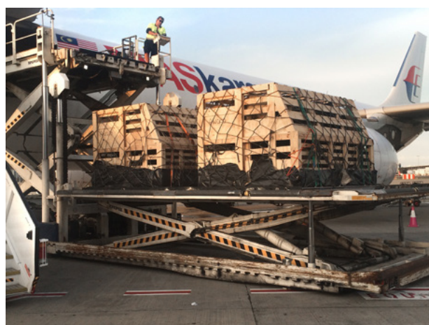
Figure 43. Livestock crates being lifted with a scissor lift to the main deck cargo door on a freighter aircraft.
