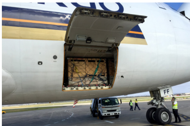
Figure 13. Loading cattle into the forward lower deck hold on a 747-400 freighter.
