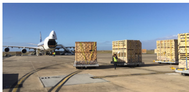
Figure 42. Livestock crates parked on the tarmac ready to load onto the aircraft. Crates should be towed onto the tarmac just before they need to be loaded on the aircraft.
