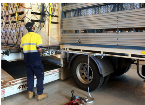
Figure 33. The aircraft crate and truck are strapped together to prevent the crate being pushed away, creating a gap that might cause injury or allow an animal to escape.
