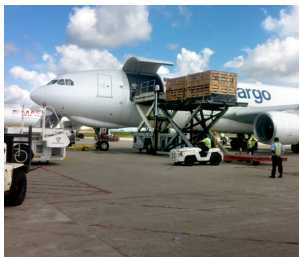
Figure 7. Unloading livestock crates from the main deck of an A330-200F freighter.
