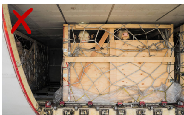
Figure 17. Cattle in a lower cargo hold. There is very little space between the top of the crate and the cargo hold roof. Open space at the top of the crate allows air flow over the cattle. However, without ventilation openings in the lower half of the crate, there is a large volume of ventilation dead space (still air) within this crate.
