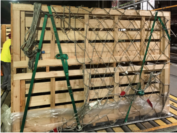
Figure 32. A double-deck sheep crate ready for loading with livestock – strapped to the pallet base and with the cargo net three-quarters of the way around the crate, leaving access to the crate door.
