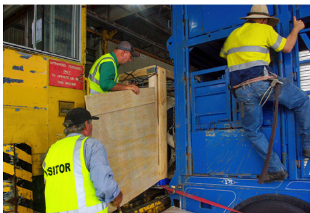
Figure 19. A crate door that slides from the side allows good control and is safe to use.
