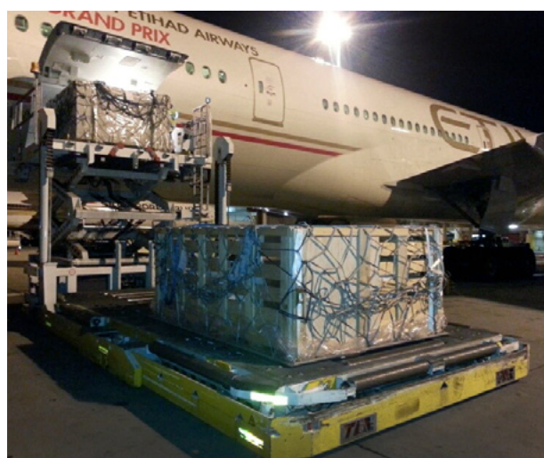
Figure 5. Livestock crates being loaded into the lower cargo hold of a passenger aircraft.
