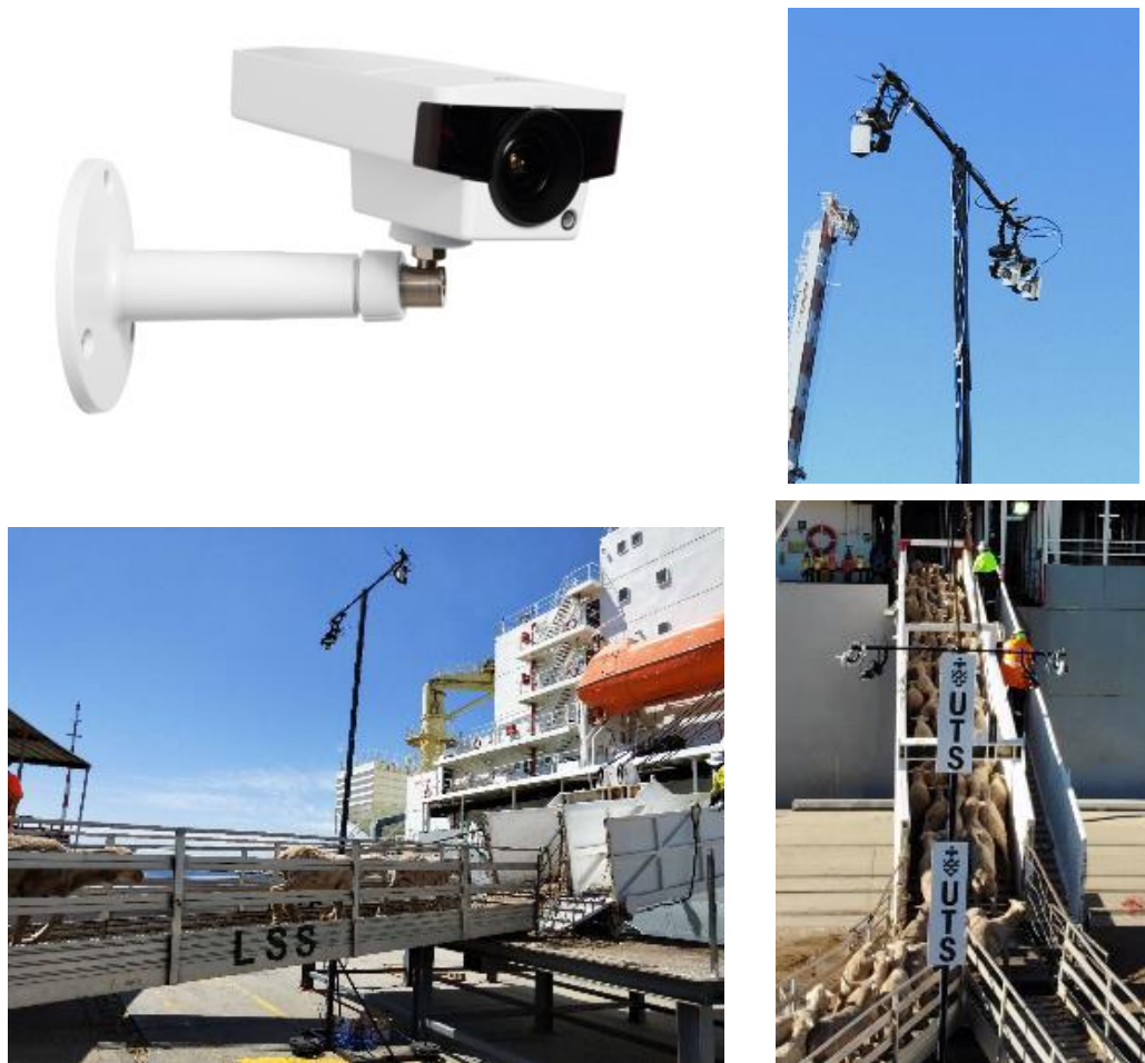
Fig. 3. Illustration of hardware design including two cameras covering two races.
