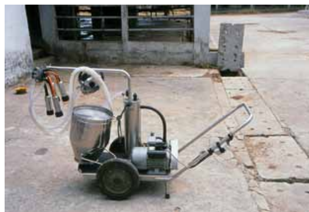
A self-contained milking machine with an electric motor can be used to keep milk from a contaminated cow entering bulk milk storage.
