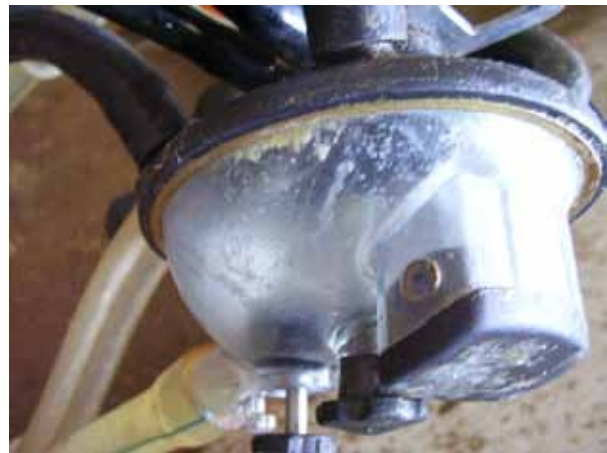
Clots of milk in this collection bowl indicate that the previous cow had mastitis which would contaminate other cows. Ideally cows with mastitis are milked last so that the bacteria are not transferred to clean cows. Cleaning equipment will avoid spreading mastitis.
