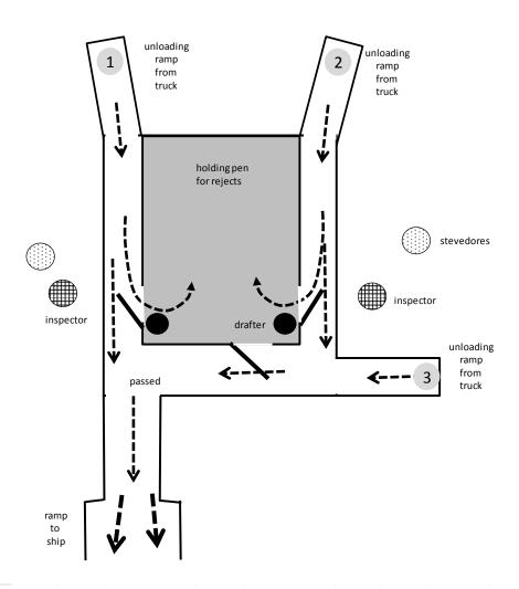
Figure 5: Depiction of a single trailer platform configured to allow for three trucks to unload through a single trailer system. Observed in action at Fremantle port.
