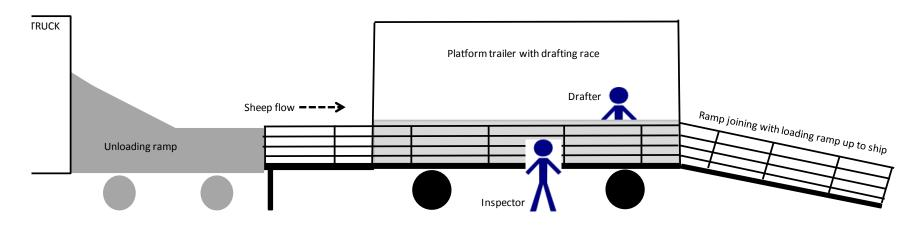
Figure 3: Lateral depiction of trailer based platform used at Fremantle wharf for individual animal inspection
