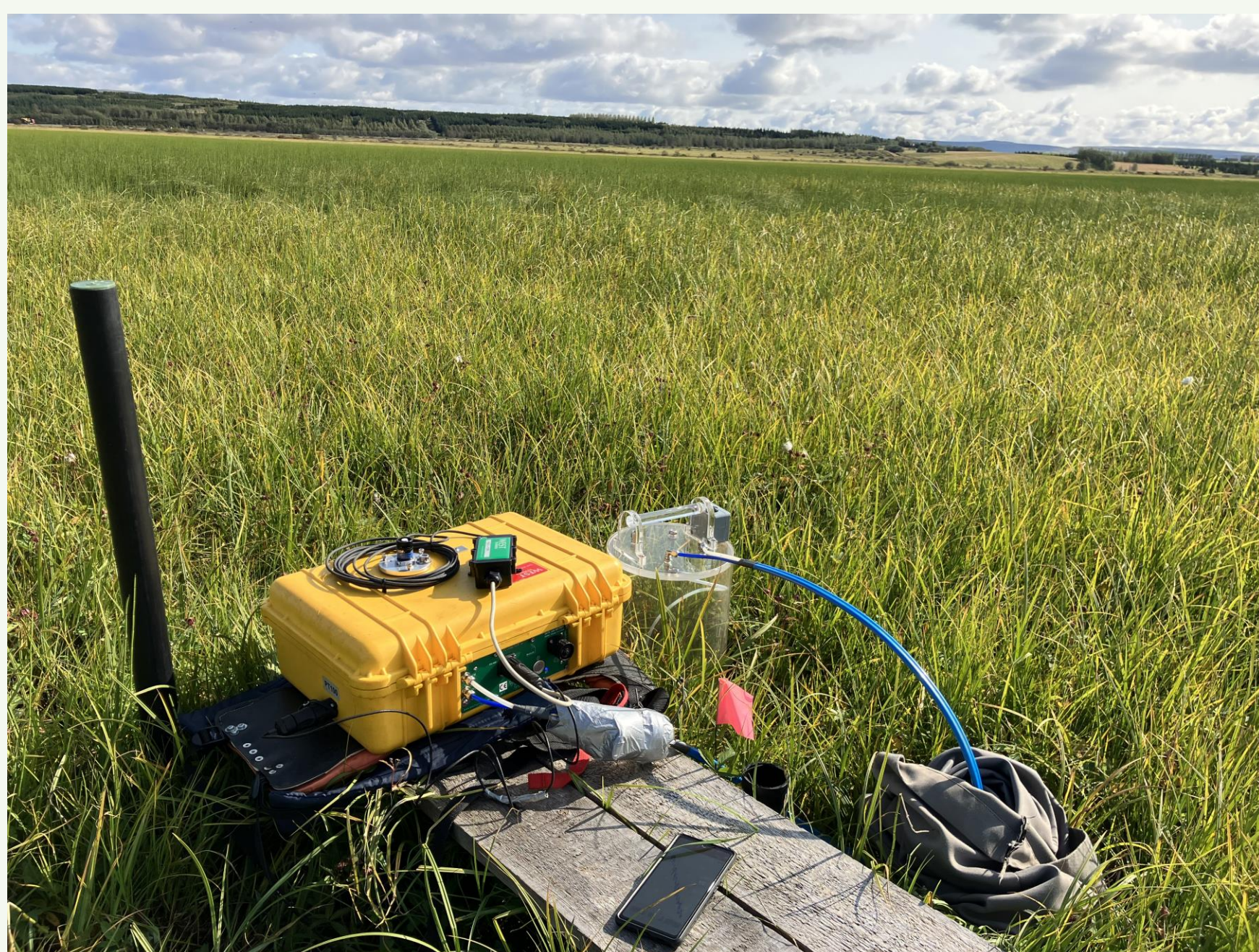
Figure 2. Monitoring site in undisturbed Carex lyngbyei fen, SW Iceland. Each has a dipwell for water table observations and three collars on which a portable soil fluxmeter may be placed. R_{ECO} is measured by covering the chamber with a light-blocking material in order to exclude primary production.
