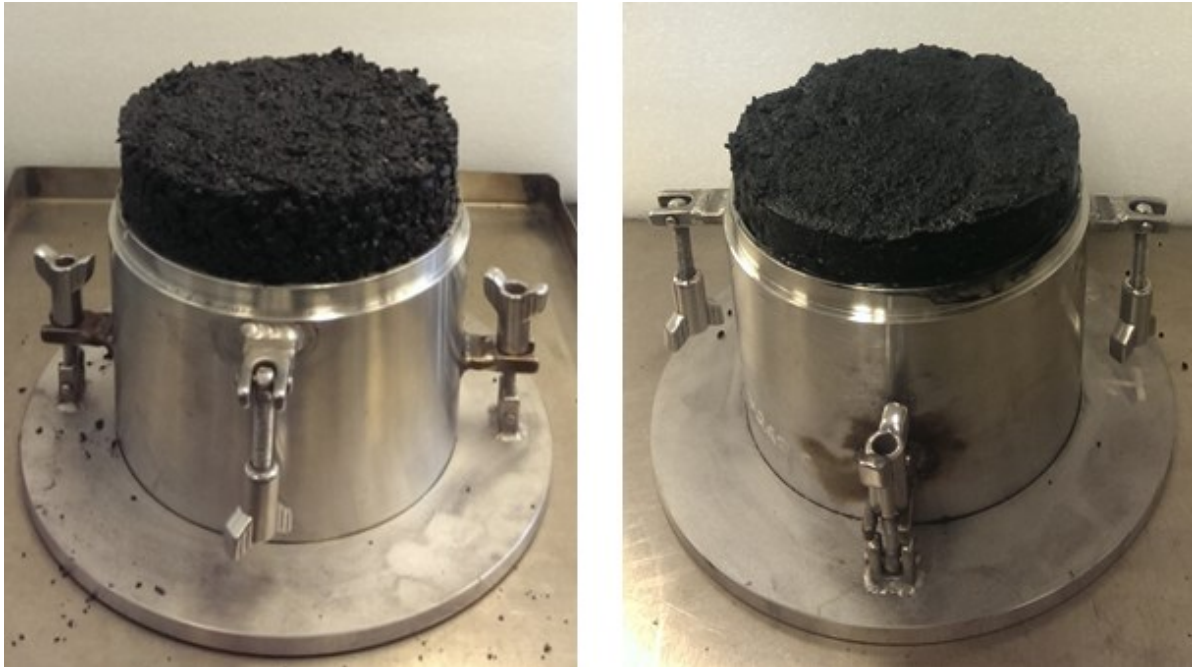
Figure 1.5.7 Photographs showing valid tests for a partially saturated test portion (left) and a near fully saturated test portion (right)
