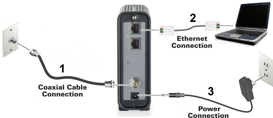
Figure 4: CM8200 Connection Diagram
