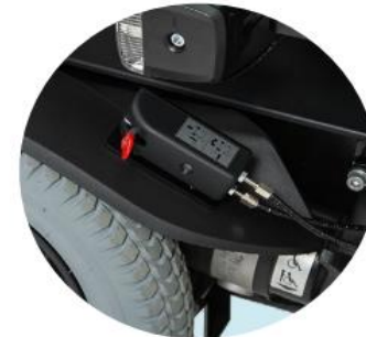
EF020 Caster wheel swivel lock
