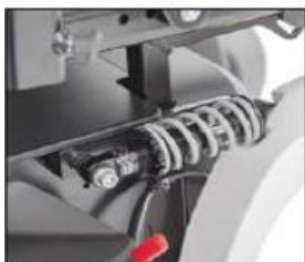
EF001 Caster wheel swing arm, spring-mounted
