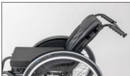
MD10 Back support, angle-adjustable
