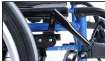
MH10 Knee lever wheel lock extension
