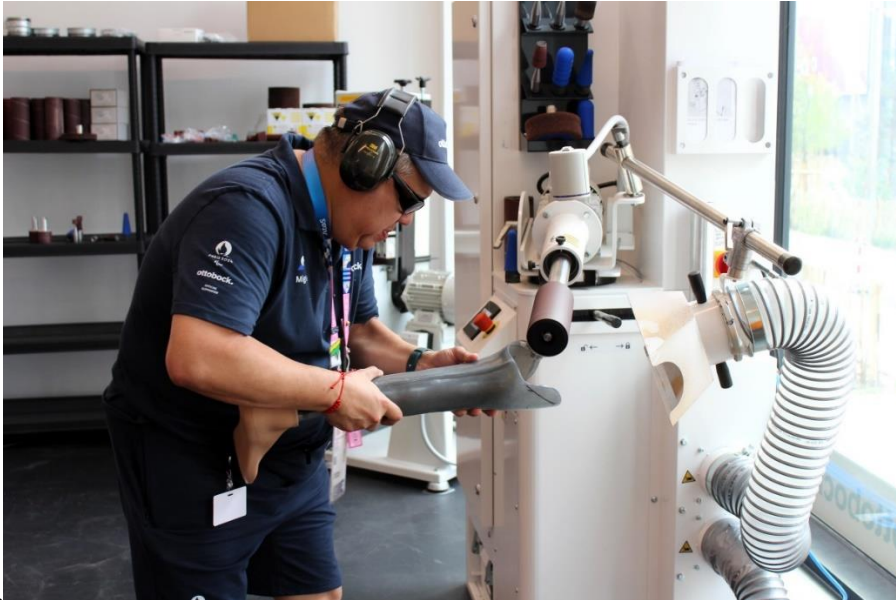
To avoid pressure points from the prosthesis, one of the technicians grinds the edge of the socket. (c)Ottobock
