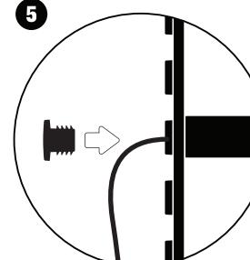
**5 Insert the cable stop to secure the cable(s)**
