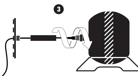
**3 Screw the tube onto Cell Alpha**
