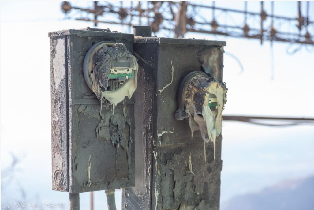
A melted electric meter box at Mount Wilson. Photo courtesy of Steve Rhoades, KABC(TV) broadcast systems specialist.
