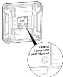
The first step in setting the advanced configuration is to remove ZEN from the wall, turn it over so the rear of the display is accessible, then press the CONFIG button *5 times*.
