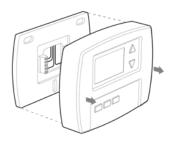
Most thermostats allow you to remove the main unit and provide access to a wall plate which holds the wiring terminals.
