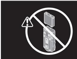
Do not install battery pack yet. The lock will not work properly unless you read and follow all instructions in step 21.
