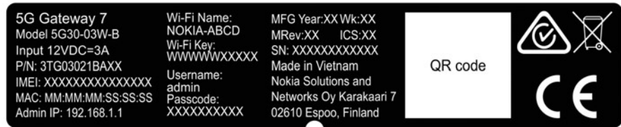
Figure 8 Example of the product label for the FastMile 5G Gateway 7 in the European and Oceania markets
