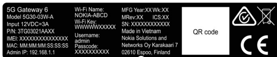
Figure 7 Example of the product label for the FastMile 5G Gateway 6 in the European and Oceania markets
