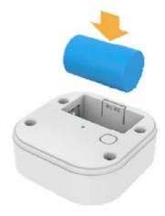
7. Insert CR2 Battery paying special attention to the battery polarity
