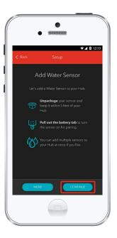
4. Prepare your Water Leak Sensor to be paired following the simple instructions on your screen. For more detailed instructions, you can tap More. 5. Once the Water Leak Sensor is detected you will see the **Sensor** icon, and **Pairing...** will appear.
