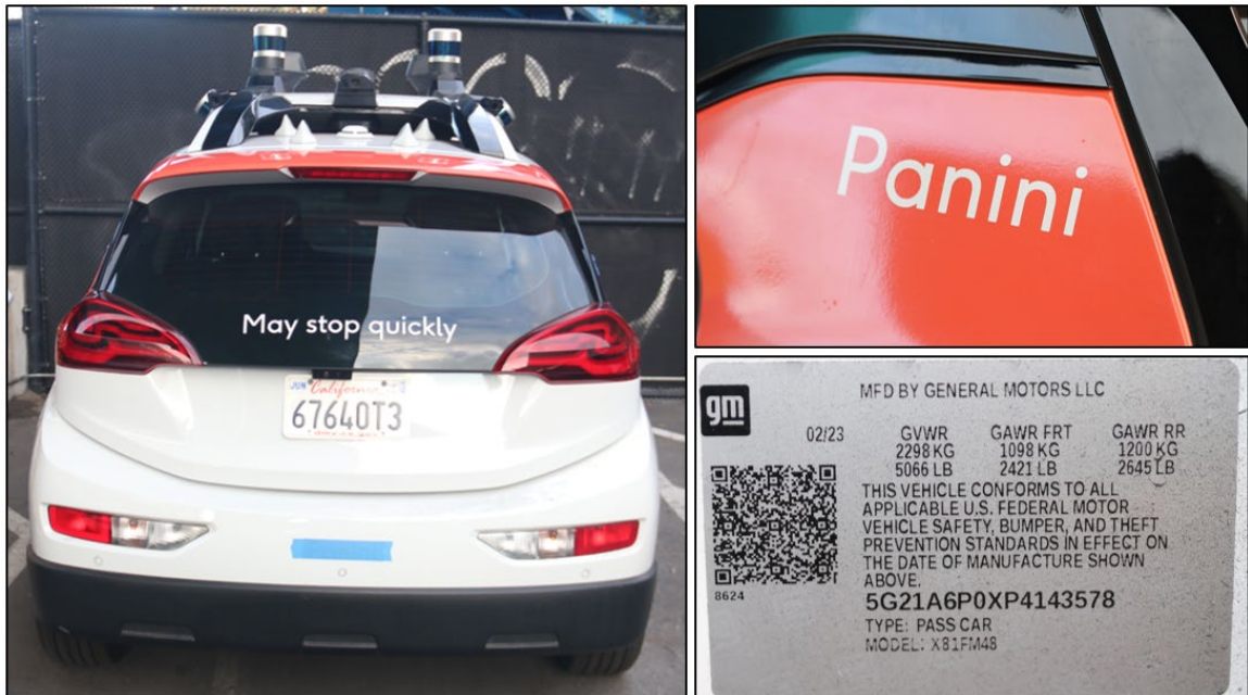
Figure 3. Photographs showing the rear of AV (left), vehicle moniker label on left side C-pillar (top-right), and vehicle VIN sticker (bottom-right). 5
