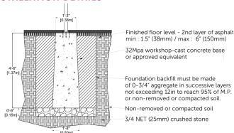
The base should be approximately level with the first layer of asphalt. All bases of the same product must be at the SAME LEVEL.
