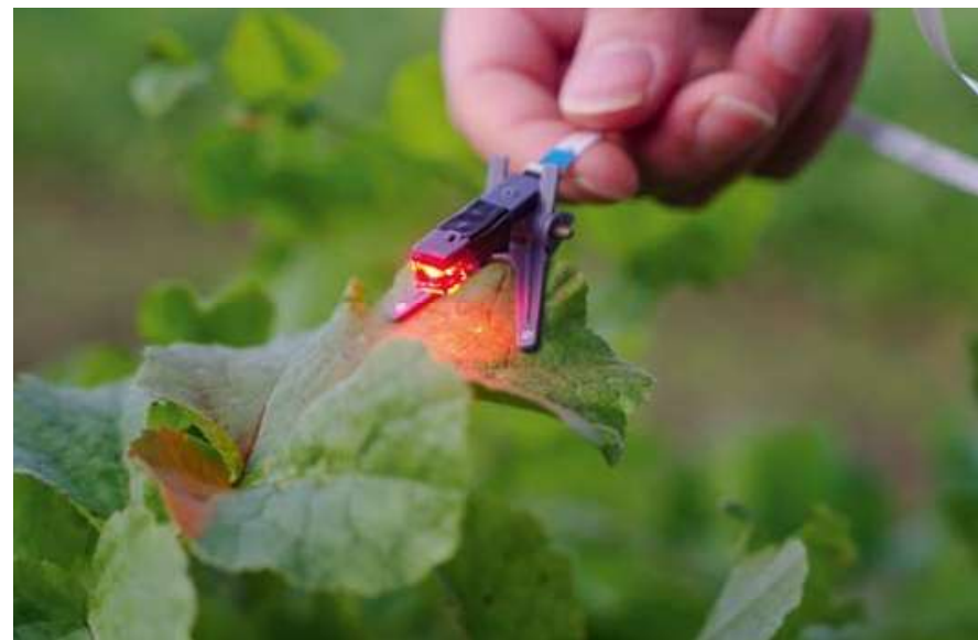
Prototype of a new sensor to make continuous photosynthesis measurements, developed by JII together with Michigan State University
