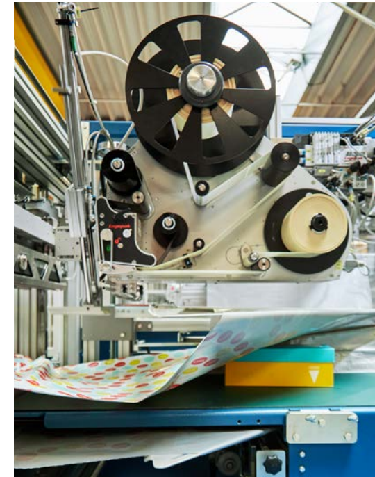
The bag packaging machine uses optical components to detect the size of a product, cuts the required film, welds it to size and prints out the label.
