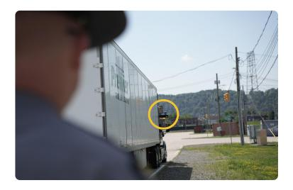
A quick flashing amber light on the sensor pod, located above the side mirrors, will indicate from a distance that the vehicle is clear to approach.
