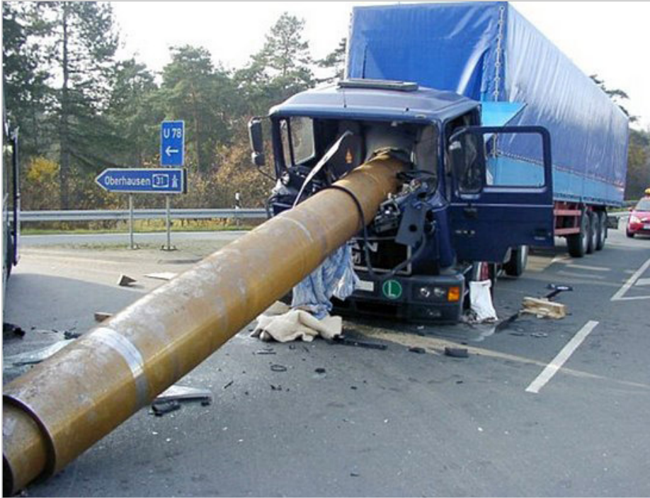
Figure 1 [Ridder] Seventeen tonnes of steel pipes inserted inside one another. Simply a braking maneuver, i.e. normal acceleration. (Photo of the month - February 2003)
